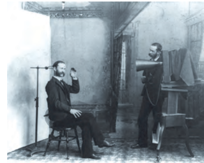
An 1850s portrait studio with a method to hold the head still during the relatively long exposure—probably several seconds.
